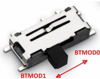
Shown positions set the corresponding BTMOD0/1 line to low. BTMOD0 controls the CPU configuration port PC9, i.e. BOOTMOD(0), while BTMOD1 is connected to the CPU configuration port PC10, i.e. BOOTMOD(1).
